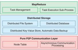
Figure 4: Outline of DDD Internal Structure
