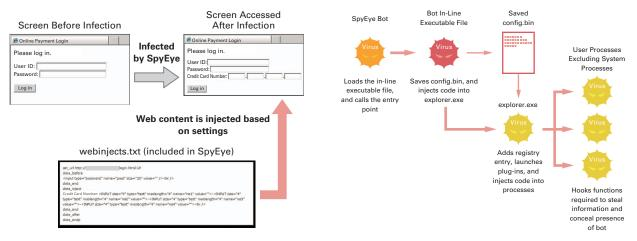
Figure 17: Example of Web Injection Using SpyEye
