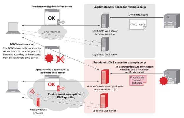
Even if a certificate authority system is hacked and a fraudulent certificate issued for www.example.co.jp, an attack is not possible unless a server is actually placed under the target domain or the DNS is also manipulated by some means. This figure is an example of circumventing the FQDN check using DNS spoofing.
