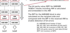
Figure 4: Relationship Between Sender/Recipient Lanes During Lane Multiplexing/Demultiplexing
