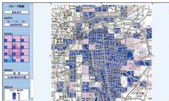
In Internet vehicle experiments conducted by the WIDE Project in Nagoya in 2001, location, speed, and wiper usage data was collected from 1,570 taxis. The blue parts of the map indicate areas with a high ratio of wiper usage, showing rainfall in detail.
