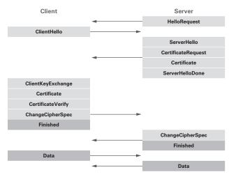
Figure 8: Certificate-Based Client Authentication Using TLS 1.2
