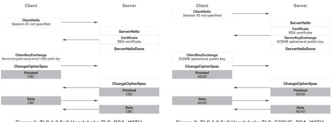
Figure 1: TLS 1.2 Full Handshake TLS\_RSA\_WITH\_ AES\_128\_CBC\_SHA
