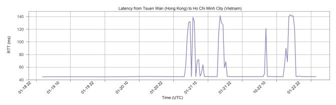
Figure 12: Latency between Hong Kong and Vietnam during Asia-America Gateway (AAG) cable reconfiguration (January 2018)
