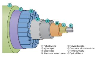
Figure 2: Cross Section of Submarine Cable with Multilayer Protection
