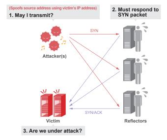
Figure 4: Overview of a SYN/ACK Reflection Attack
