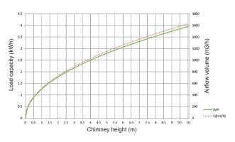
Figure 10: Chimney Effect Test Results (excerpt: change in airflow volume according to chimney height)
