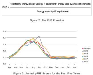
high-power-consumption mode that does not use outside air. In comparison, spring and autumn pPUE readings are around 1.1 because the modules run in a low-power mode that uses outside air. In winter, the modules mix IT equipment exhaust and outside air to achieve the right temperature, and since this mode also consumes less power, pPUE is around 1.1. The average over the past five years is 1.18.
