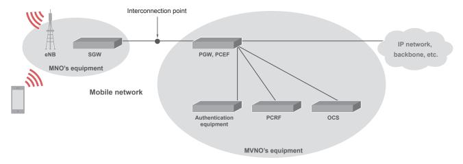
Figure 10: Connection Sequence from Mobile Phone to MVNO Network
