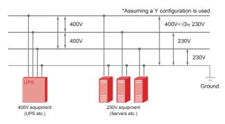
Figure 7: Y-connection Overview of Three-phase Four-wire System
