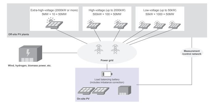
Figure 19: Carbon-Neutral Data Center Model
